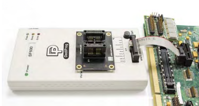
Fig 3: SF600 connected to the application header
