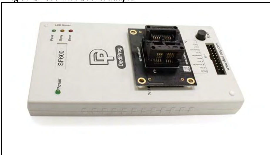
Fig 5: SF600 with Socket adaptor
